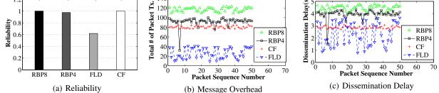
Figure 14. The Performance of Outdoor Linear Network Experiment
