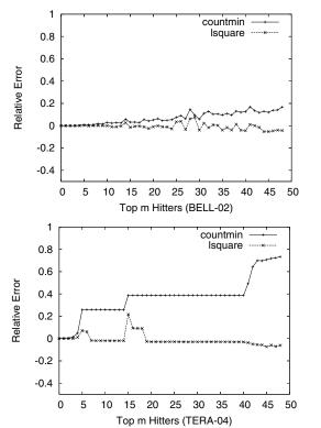
Figure 2: K = 1024, H = 4, m = 50: Isquare shows more accurate and stable estimation than countmin.
