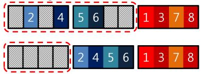
Four live blocks should be moved to secure an empty segment.
