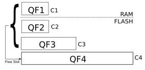
Figure 1: Cascading Filter
