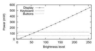
Figure 14: Display, button and keyboard backlight power on the G1.
