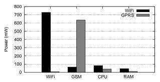
Figure 7: Power consumption of WiFi and GSM modems, CPU, and RAM for the network microbenchmark.
