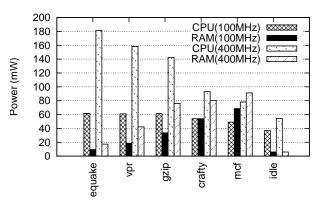
Figure 5: CPU and RAM power when running SPEC CPU2000 micro-benchmarks, sorted by CPU power.
