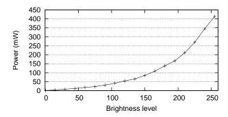
Figure 4: Display backlight power for varying brightness levels.
