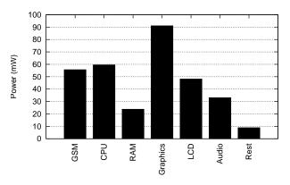
Figure 8: Audio playback power breakdown. Aggregate power consumed is 320.0 mW.
