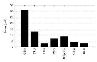
Figure 2: Power breakdown in the suspended state. The aggregate power consumed is 68.6 mW.
